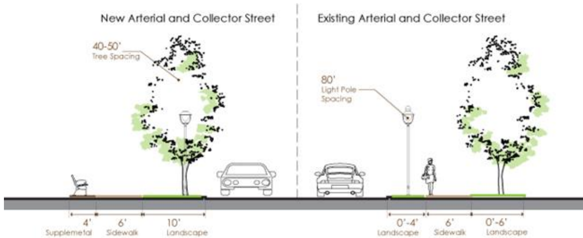
Streetscape Figure—Arterial and Collector Streets
