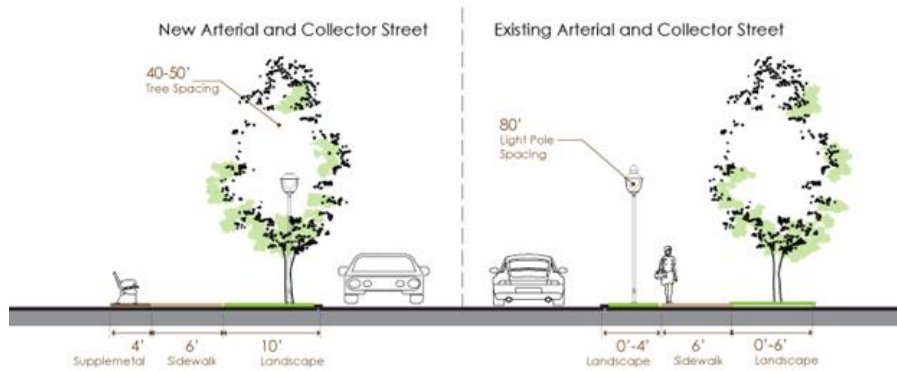
Streetscape Figure—Arterial and Collector Streets
